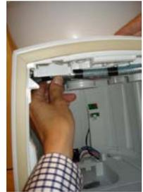
**H** Rotate the retainer back in position
