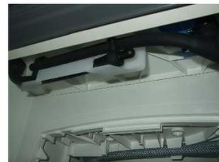
You have now completed the fitting of the additional drain tube. Please note that there still may be some water in the tank and therefore we advise if this is not the final destination of the vehicle before it goes into storage that both the drain tubes are opened and emptied again to remove any water which may have moved during transit. This will eliminate the chance of any water causing frost damage to the pump.
