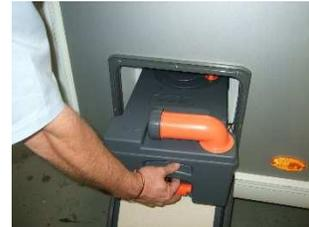
Remove the waste holding tank and pull out the drain tube from its retaining bracket.
