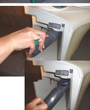
Press new waterfill funnel in. Note: first push the rear of the funnel in position then pull the front up.
