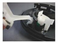
Place complete mechanism back and use sliding cover in reverse to position complete mechanism back into the tank.
