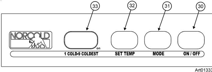
The refrigerator control panel (See Art01333) is between the freezer compartment and the fresh food compartment. To maintain the operating control functions of the refrigerator, a 12 volt DC power supply is necessary. The refrigerator receives DC power from the 12 volt system of the vehicle; either an auxiliary battery, a converter, or the vehicle engine battery.
